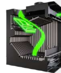
SMOKE BY-PASS ON
